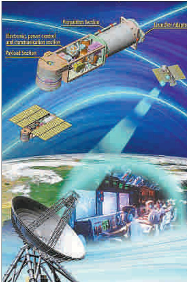
**Efficient and Endurable:** Rafael's planned LiteSat-B, pictured in an illustration from a company brochure, is intended to use solar-generated electric thrust instead of conventional chemical thrusters to move about in orbit.
